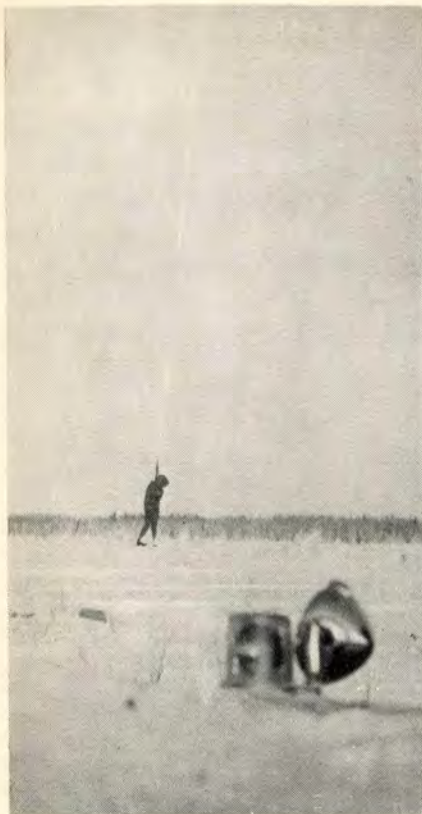
Dummy attached to lift line begins journey aloft, reaches aircraft ramp in photo at right.
